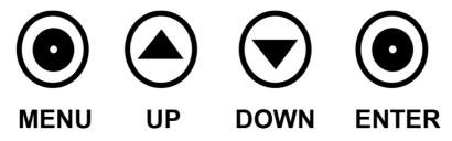
Please press the "MENU" to exit or return to the previous menu, press "UP" or "DOWN" to select the upper and lower menus or adjust the values, and press "ENTER" to confirm.
