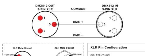
Pin1: Ground pin2: Negative pin3: Positive
