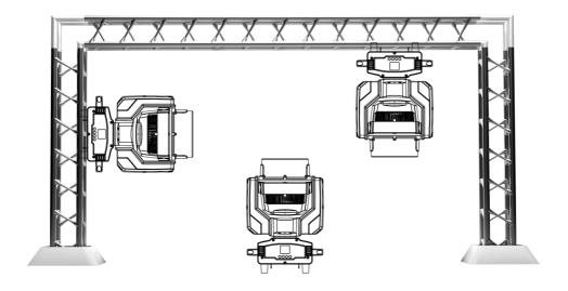
740BW works properly in above different mounting, hanging upside-down from a ceiling, sideways on trussing, or set on smooth horizontal surface. Be sure this facility is at least 12m (40ft) away from flammable materials (decoration
