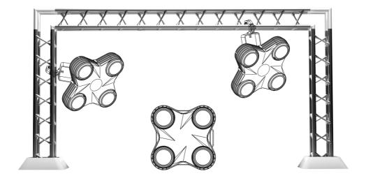
4200LW works properly in above different mounting, hanging upside-down from a ceiling, sideways on trussing, or set on smooth horizontal surface. Be sure this facility is at least 12m (40ft) away from flammable materials (decoration etc.). Always use and install the safety cable to prevent accidental
