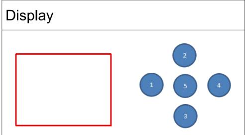
Please press the "ESC" to exit or return to the previous menu, press "UP" or "DOWN" to select the upper and lower menus or adjust the values, and press "ENTER" to confirm.
