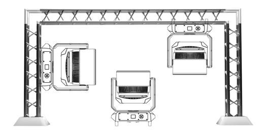
1960BW-4 works properly in above different mounting, hanging upside-down from a ceiling, sideways on trussing, or set on smooth horizontal surface. Be sure this facility is at least 12m (40ft) away from flammable materials (decoration etc.). Always use and install the safety cable to prevent accidental damage or injury from the facility failure. Never use handles for secondary attachment.
