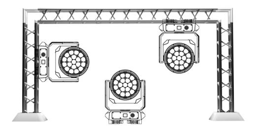
1940BWR works properly in above different mounting, hanging upside-down from a ceiling, sideways on trussing, or set on smooth horizontal surface. Be sure this facility is at least 12m (40ft) away from flammable materials (decoration etc.). Always use and install the safety cable to prevent accidental
