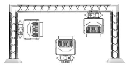
1940B MINI IP works properly in above different mounting, hanging upside-down from a ceiling, sideways on trussing, or set on smooth horizontal surface. Be sure this facility is at least 12m (40ft) away from flammable materials (decoration etc.). Always use and install the safety cable to prevent accidental damage or injury from the facility failure. Never use handles for secondary attachment.
