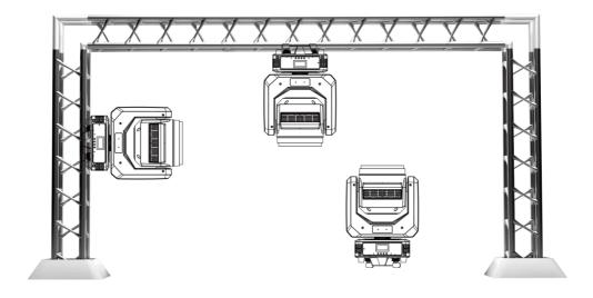
1920Z works properly in above different mounting, hanging upside-down from a ceiling, sideways on trussing, or set on smooth horizontal surface. Be sure this facility is at least 12m (40ft) away from flammable materials (decoration
