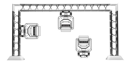
1240B works properly in above different mounting, hanging upside-down from a ceiling, sideways on trussing, or set on smooth horizontal surface. Be sure this facility is at least 12m (40ft) away from flammable materials (decoration etc.). Always use and install the safety cable to prevent accidental damage or injury from the facility failure. Never use handles for secondary attachment.
